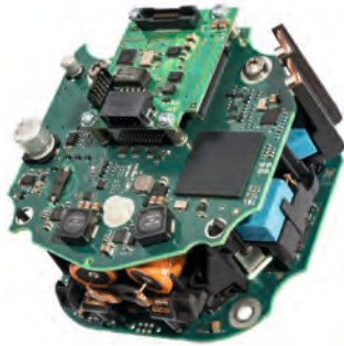
Control device to regulate the motor of the Intelligent eQualizer in the pro-active chassis of the new Mercedes-Benz GLE
