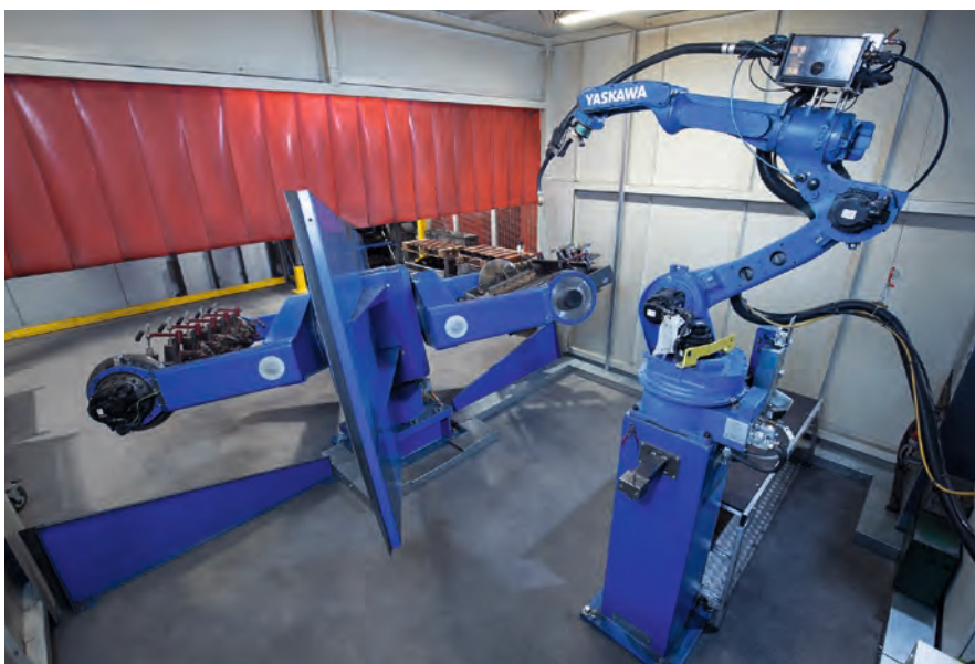
YASKAWA's five-axis, 2-station positioner enables loading on the one side and welding on the other.
