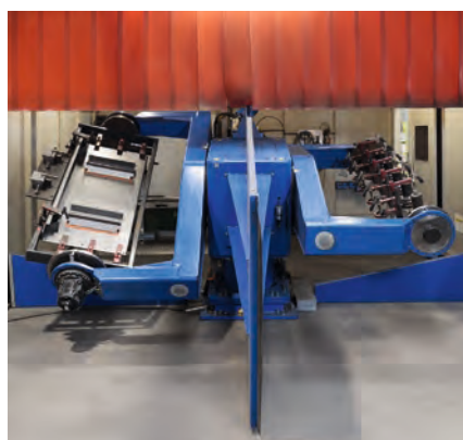
Imposing: the YASKAWA R2C five-axis servo positioner with two stations for parallel loading and welding.
